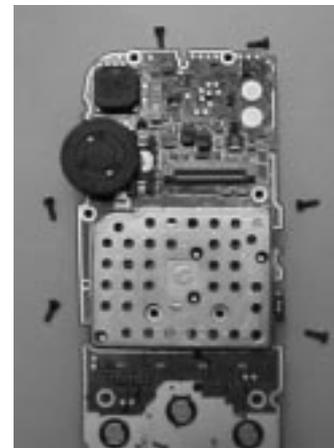
8. Remove 6 screws located on the display side to release the patch antenna.
