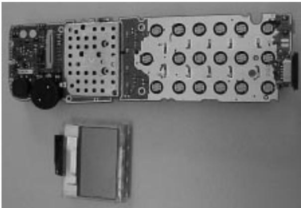
7. The display unit can be lifted out. The LCD is connected with a flex cable and the LCD support is clamped onto the main board (2 clamps left and right side).
