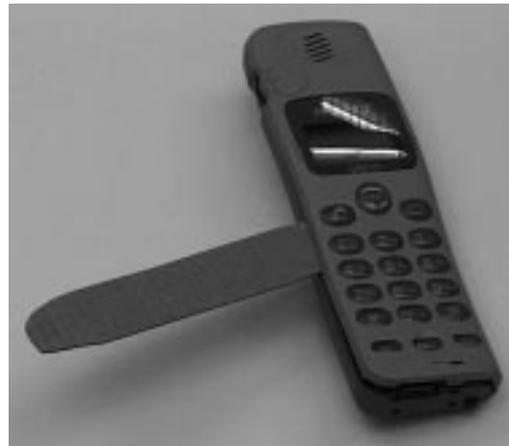
3. The lower claws can be released by gently pushing the upper case to left/right versus the lower case.
