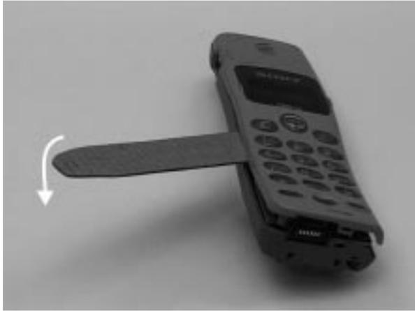
5. Push the hook release jig gently to the lower side, while holding the CMD-C1. In this way the hook release jig is used as a lever. More clamps between upper and lower case will now release and the parts can be taken out.
