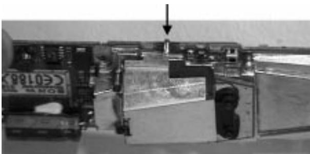
9. Unsolder the antenna on the right side. The patch antenna assy can now be lifted off. It should be considered as one non-serviceable and sensitive item.
