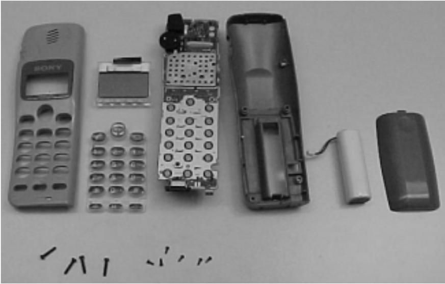
10. Parts on the main board specified in the parts list can now be reached.
