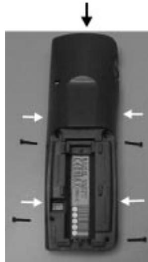
1. Remove the battery cover and the battery. Note that the SIM card is also located in this area.
